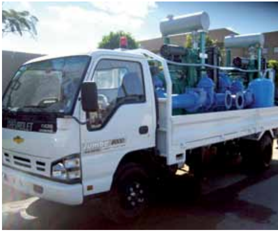
Mobile response unit carrying water pumps powered by Cummins G-Drive engines.
